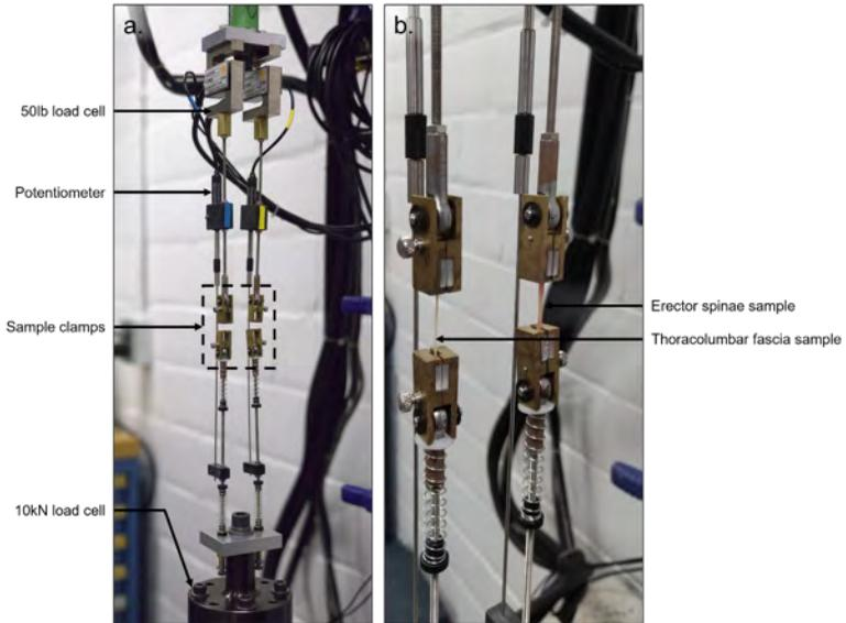
Figure 1: Custom-built apparatus used for individual and dual tension testing of cadaveric samples (a) without samples undergoing testing and (b) with thoracolumbar fascia and erector spinae samples inserted.
