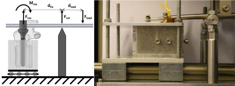
Fig.1: Experimental setup designed to mimic *in vivo* loading of spinal fixation members. By applying a compressive force onto an instrumentation rod, positioned over a hinge point, a pull-out force and moment are applied to the fixation member. An excess of shear forces was avoided by mounting the specimen on a sliding surface.
