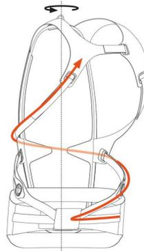
Twisted State: During an accident the RSP System tightens around the body impeding excessive rotation.
