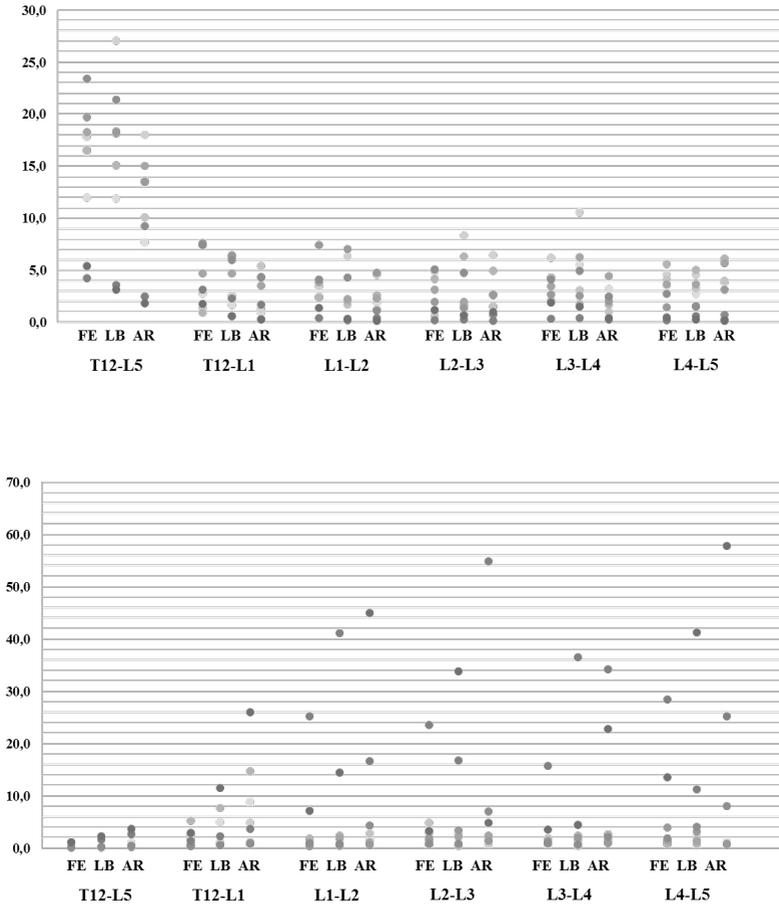
Fig. 1: The ROM (in degrees; upper diagram) and NZ stiffness (in Nm/degree; lower diagram) for each spine, for the whole spine and per segment, and per direction.
