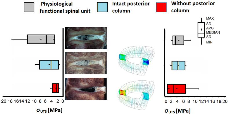
Fig. 1: Influence of the articular triad of mechanical and structural properties of the annulus fibrosus in experimental and numerical research.
