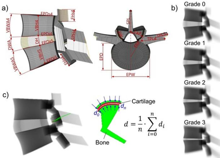
Fig. 1: a) Parametric finite element model of a human L4-L5 motion segment. b) Simulated "X-rays" (inverted) of the models representing different stages of degeneration (averaged images of individual models for each group). c) The facet joint gap is determined as the mean distance between the opposing bony surfaces of the facets in the cutting plane through the middle of the facet joint.
