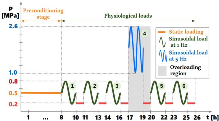
Fig. 1: Overloading regime that includes the loading/recovery periods of the test.
