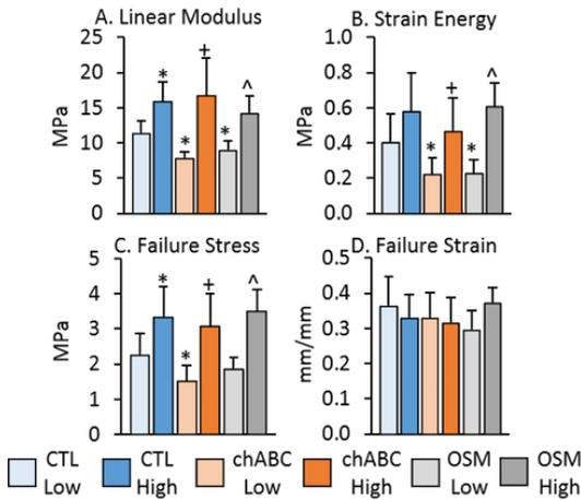
Fig. 1: Summary of mechanical properties in uniaxial tension (n = 11 per group): A) linear-region modulus, B) strain energy to the point of failure, C) failure stress, and D) failure strain. \* denotes  $p < 0.05$  vs CTL-Low, † denotes  $p < 0.05$  vs chABC-Low, ^ denotes  $p < 0.05$  vs OSM-Low in post-hoc analysis.
