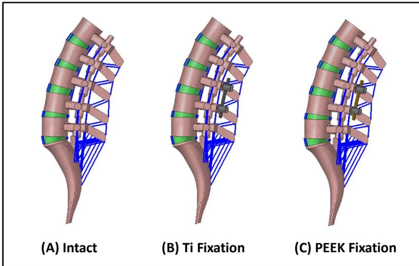
Fig. 1: Poroelastic finite element models for (A) intact, (B) Ti Fixation, (C) PEEK Fixation.
