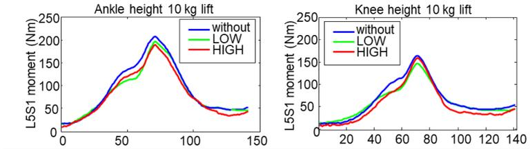
Fig. 1: Effect of two support devices on L5/S1 extension moments during ankle (left) and knee (right) height lifts, averaged over participants (N=11).
