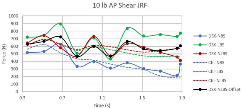
Fig. 2: Anterior-posterior (AP) shear joint reaction forces for different of the lumbar spine during sagittally symmetric lifting task with the 10 lb (4.5 kg) external weight. NBS = no bushings, LBS = linear bushings, NLBS = nonlinear bushings, PRE = preload.
