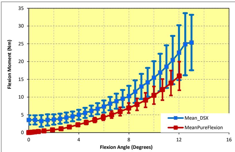
Fig. 2: FE-computed reaction moment-angular displacement (flexion) curves based on (a) Pure flexion rotation, and (b) DSX-based coupled rotation-translation kinematics.
