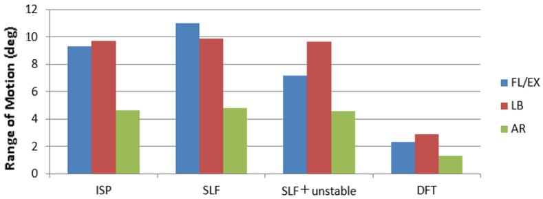
Fig. 1: L3/4 ROM of the four groups under flexion/extension, lateral bending and axial rotation; ISP, intact spine; SLF, single-level fusion in L5/S1; DFT, single-level fusion in L5/S1 and dynamic fixation in L4/5; TLF, two-level fixation in L4/5 and L5/S1.
