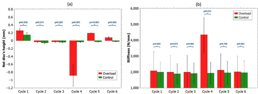
Fig. 2: Significance tests of the (a) Net disc's height and (b) axial stiffness.
