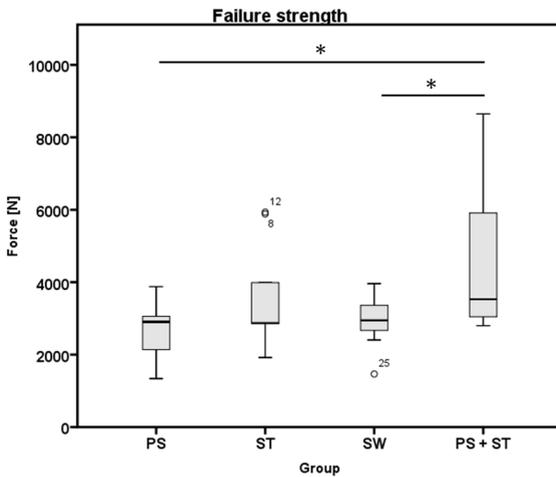
Fig. 2: The failure strength of pedicle screw constructs reinforced with sublaminar tape (PS + ST) is significantly higher compared to stand alone pedicle screws (PS) or metal sublaminar wires (SW). The pullout strength of sublaminar tape (ST) was comparable to PS and SW.
