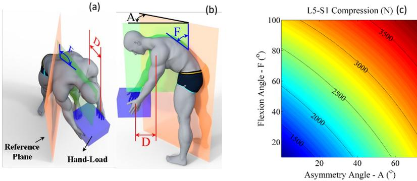
Fig. 1: (a, b) Schematic representation of an asymmetric lifting task (A: asymmetry angle; F: flexion angle; D: moment arm from the shoulder joint), and (c) contour plot of L5-S1 compression (N) computed from regression equations at hand-load weight=10 kg, D=0 cm, sex=male, body height=175 cm and body mass=75 kg.
