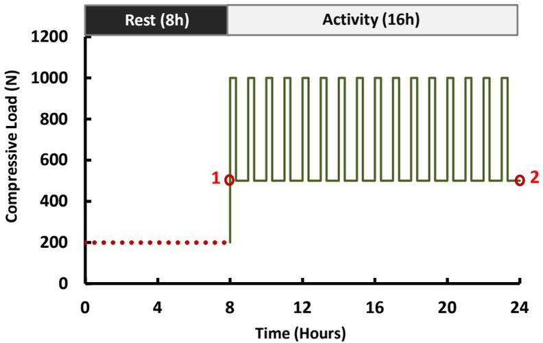
Fig. 2: Loading scenario of the compressive force (Flexion, extension, lateral bending and axial rotation moments of 10 N.m were applied at points 1 and 2).
