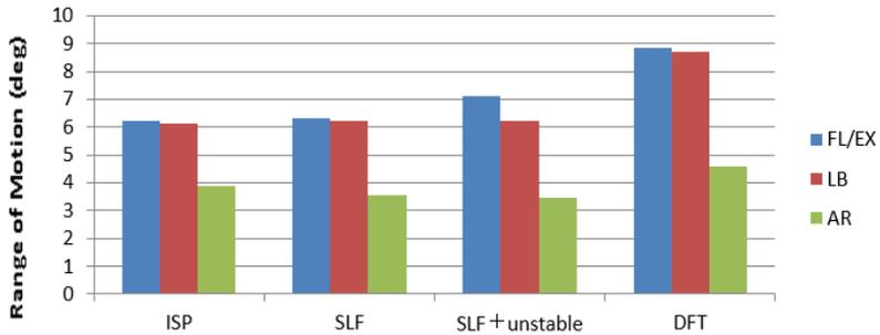
Fig. 2: L4/5 ROM of the four groups under flexion/extension, lateral bending and axial rotation; ISP, intact spine; SLF, single-level fusion in L5/S1; DFT, single-level fusion in L5/S1 and dynamic fixation in L4/5; TLF, two-level fixation in L4/5 and L5/S1.
