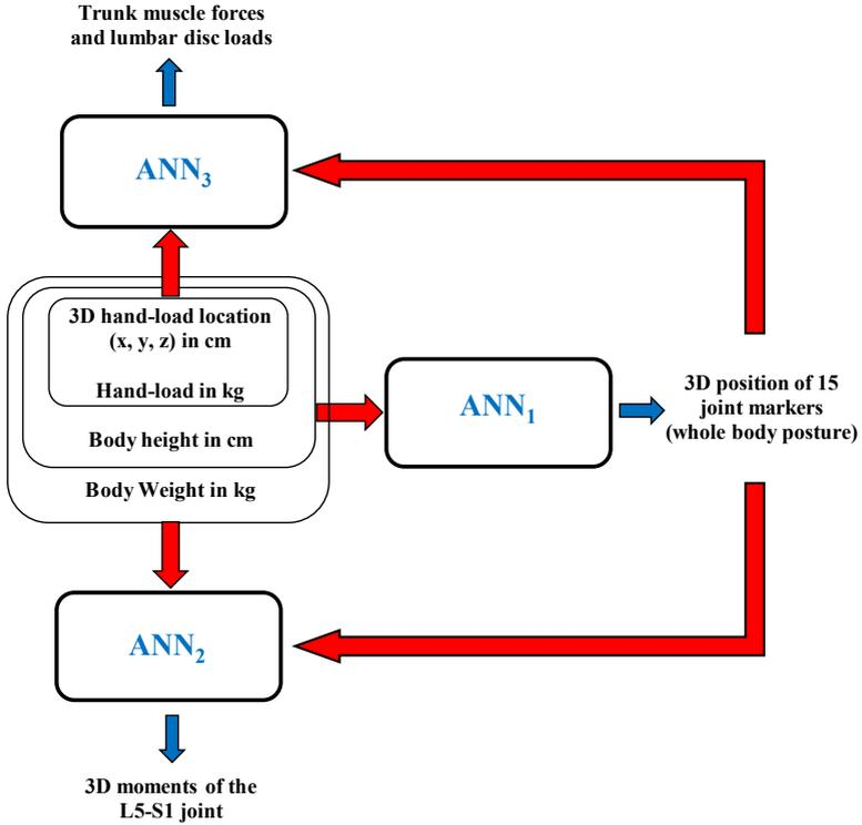
Fig. 1: A schematic of the coupled ANNs.
