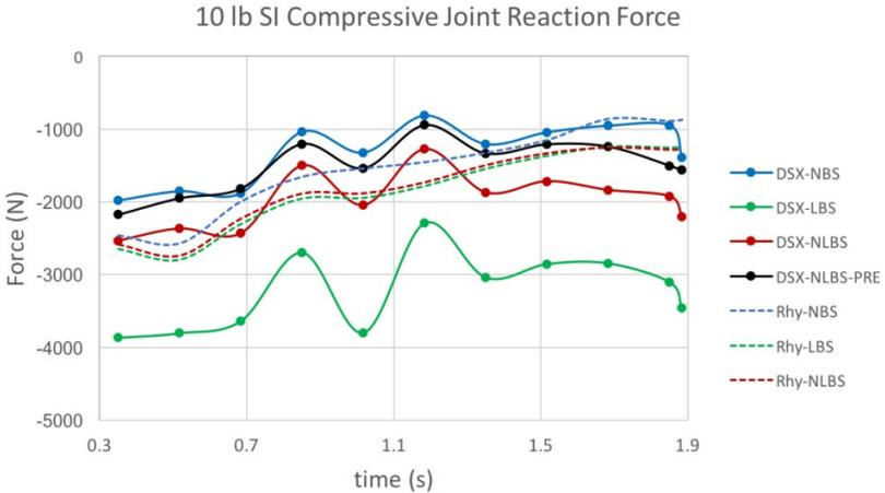
Fig. 1: Superior-inferior (SI) compressive joint reaction forces for different variations of the lumbar spine during sagittally symmetric lifting task with the 10 lb (4.5 kg) external weight. NBS = no bushings, LBS = linear bushings, NLBS = nonlinear bushings, PRE = preload.
