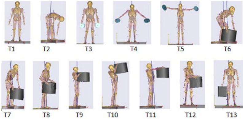
Fig. 1: Standing, flexion and 11 different loaded lifting tasks (T3 - T13) performed by each participant.
